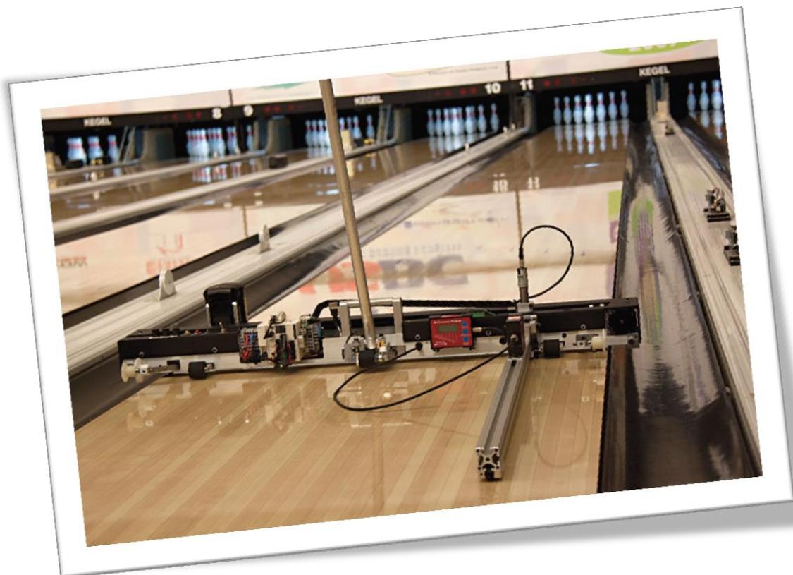
**Topography** is defined as the graphical representation of surface features indicating relative positions and elevations. It's a known fact that changes in topography adversely affect the ball path and ball motion (rate of energy depletion). When topographical features are randomly different on a bowling lane, so is ball motion.
