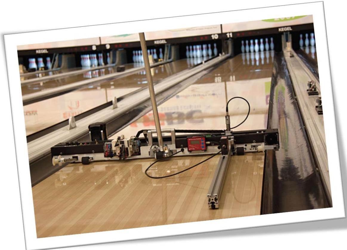
**Topography** is defined as the graphical representation of surface features indicating relative positions and elevations. It's a known fact that changes in topography adversely affect the ball path and ball motion (rate of energy depletion). When topographical features are randomly different on a bowling lane, so is ball motion which causes inconsistency.
